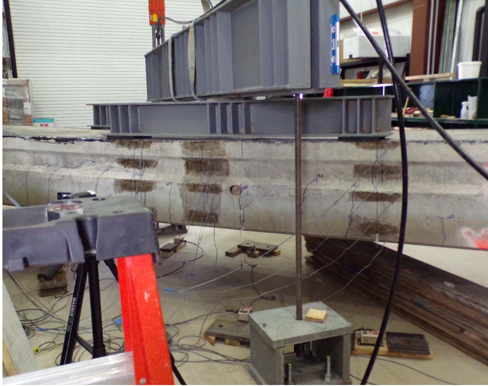
Figure 5.16: Cracking in Specimen R4 at 160 kip
