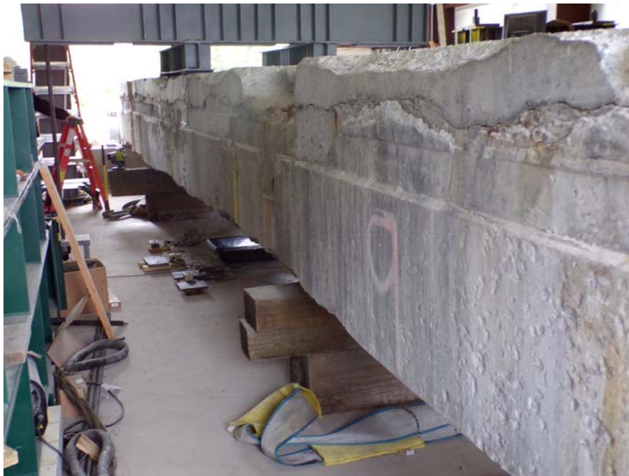
Figure 4.25: Concrete patching along top of Specimen E9
