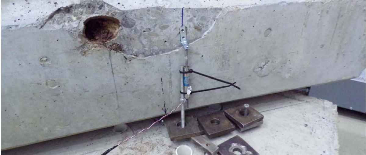
Figure 5.4: Typical attachment of potentiometer at supports
