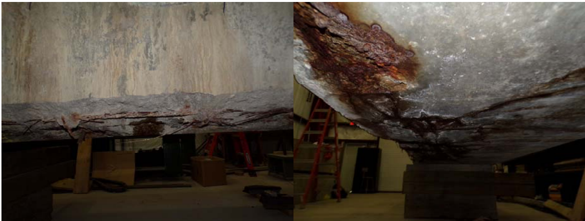
(c) View of Section 4 before and after test Figure 7.5: Deterioration of Specimen E3
