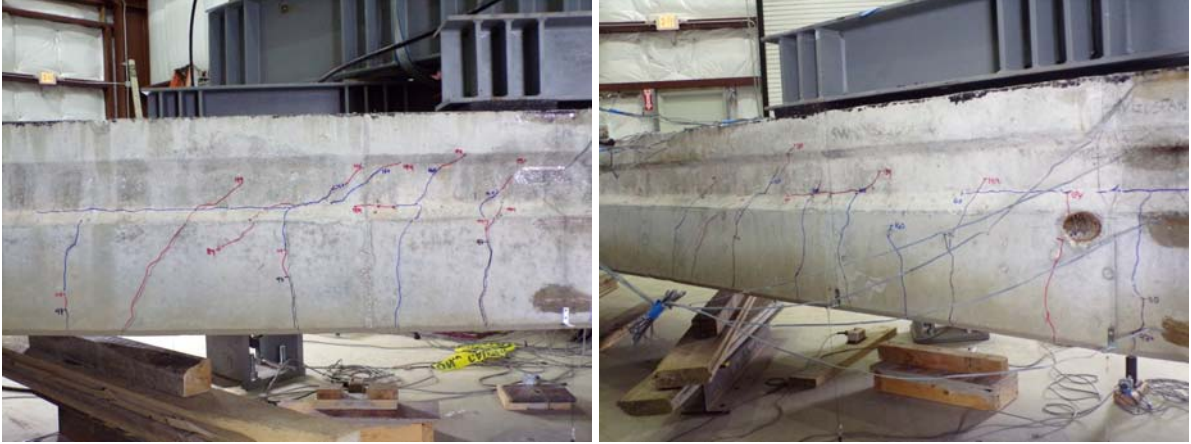
Figure 5.9: Cracking of Specimen R2 (northeast and southwest load points, 184 kip)
