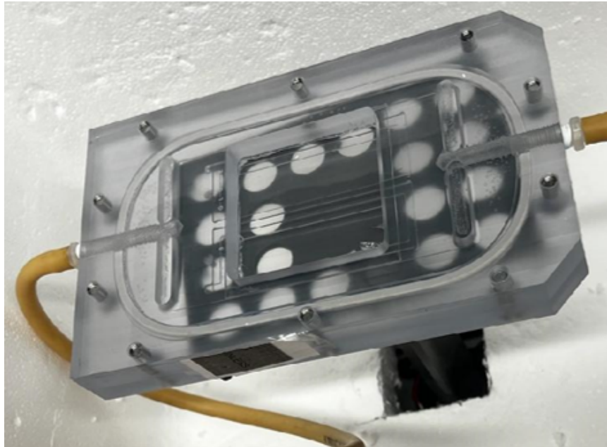
Figure 3.5: Designed PPFC in an incubator with fluid flowing through.
