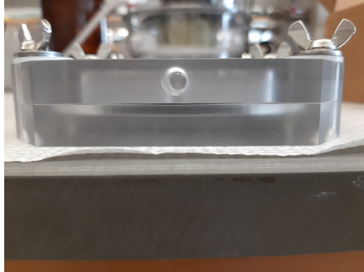
(a) Shows the slight bowing of the PPFC due to the lack of screws on the outer portion of the O-ring on the outside toward the inlet.
