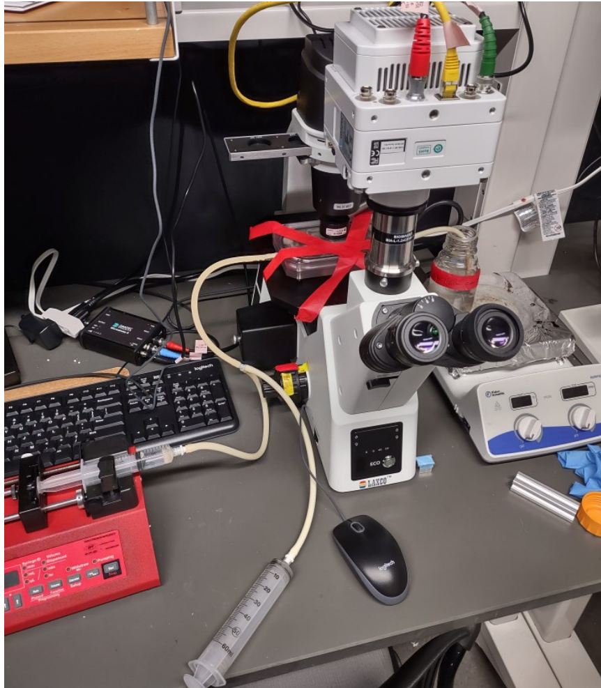
Figure 3.7: PIV setup, PPFC is taped down to avoid motion during imaging. The red device on the bottom left of the image is the syringe pump.
