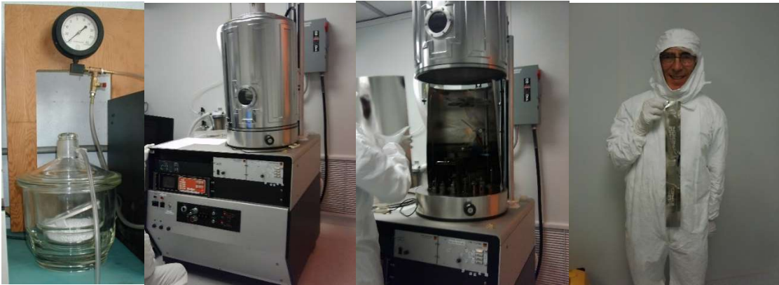
Figure 24: Coating of PET film with nickel in the SE-600 electron beam evaporator.
