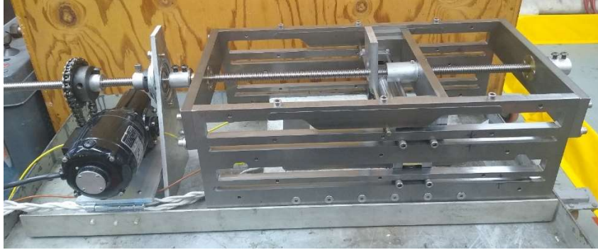
Figure 72: The roller hot embossing mechanism with wider side walls.
