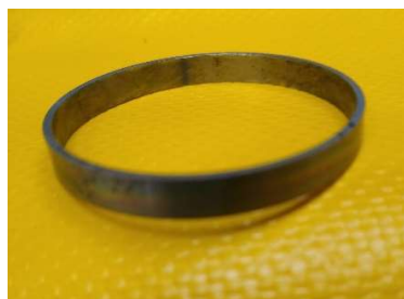
Figure 73: Mandrel roller for testing 5 mm MG rings.
