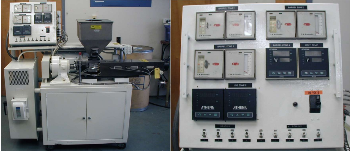
Figure 3: C. W. Brabender Type 125-25HC four zone 1.25 inch extruder and PID controllers.
