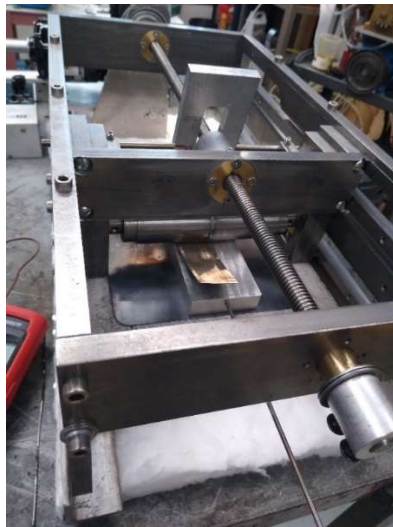
Figure 84: The nickel mold curled.
