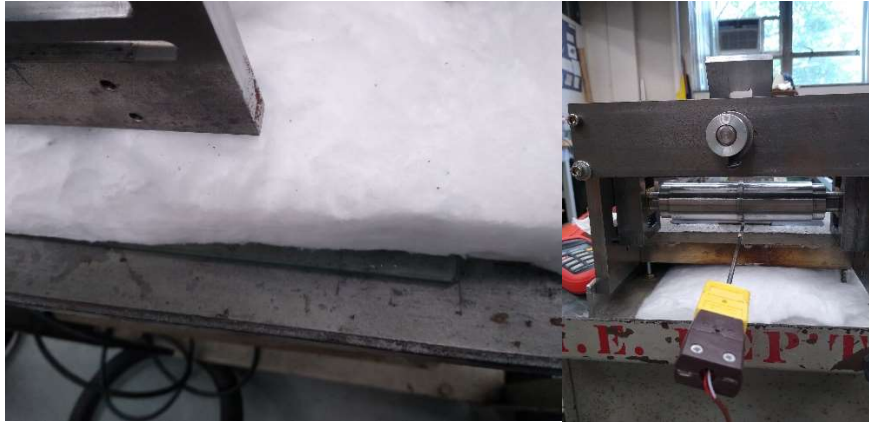
Figure 82: Glass plate and ceramic wool insulation under the hot roller embossing mechanism.
