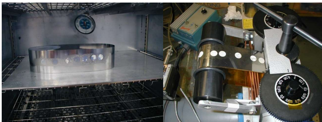
Figure 30: Curing the glue in an oven to secure Alumina filter disks to SS ribbon belt and the belt installed on the calender roll.
