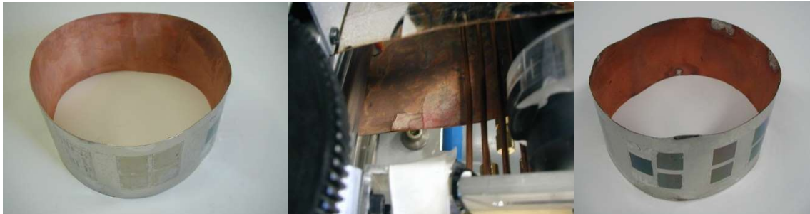
Figure 53: Belt with copper layer, cracking and delaminating, repaired with solder.
