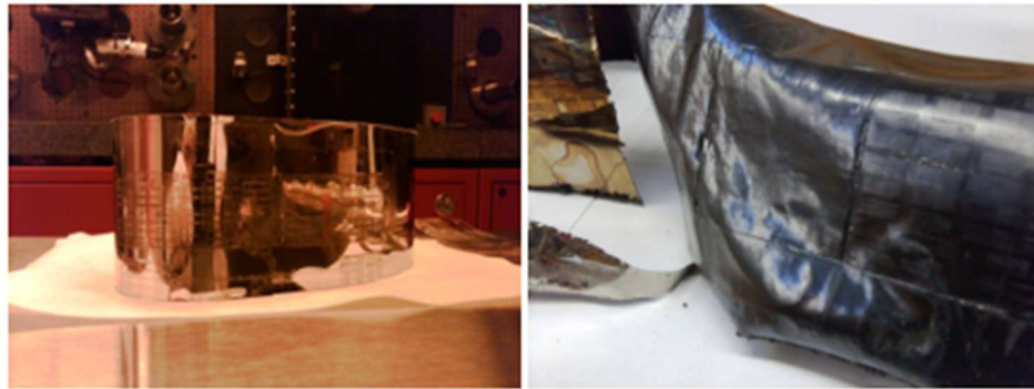
Figure 50: Mold belt before and after heat treatment in a vacuum oven.
