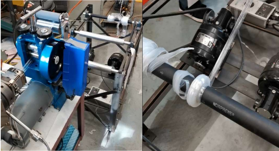
Figure 88: Path of LDPE web through the calender, over the cooling roller and to the winder.
