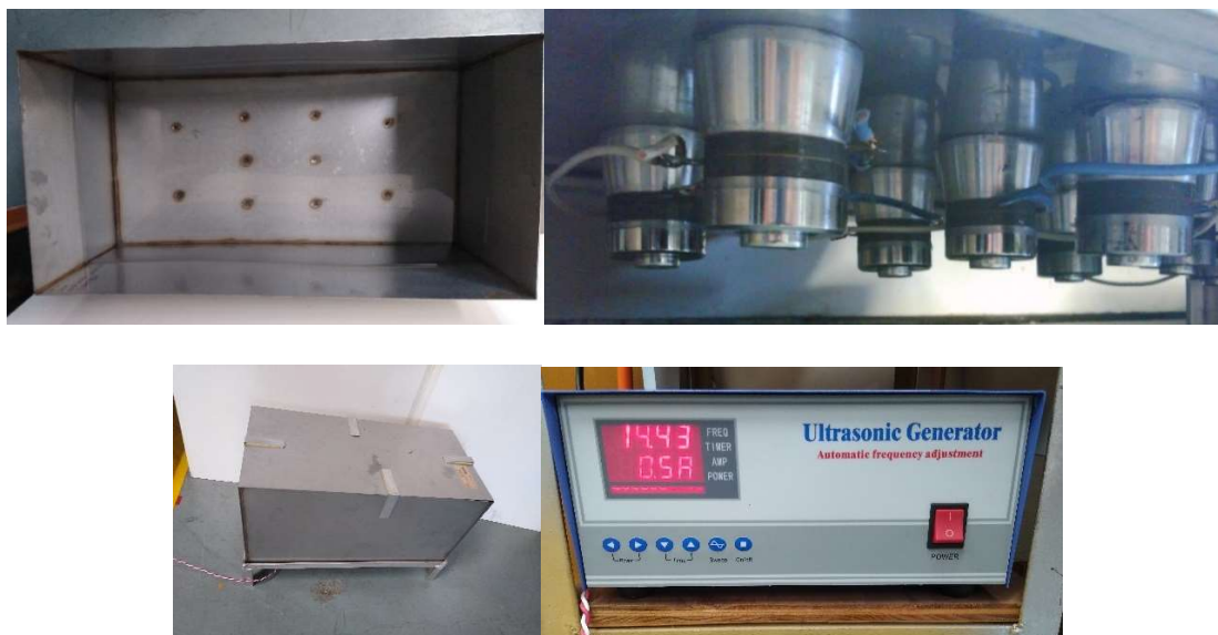
Figure 58: The ss tank with the ten 40 kHz transducers mounted on the bottom.
