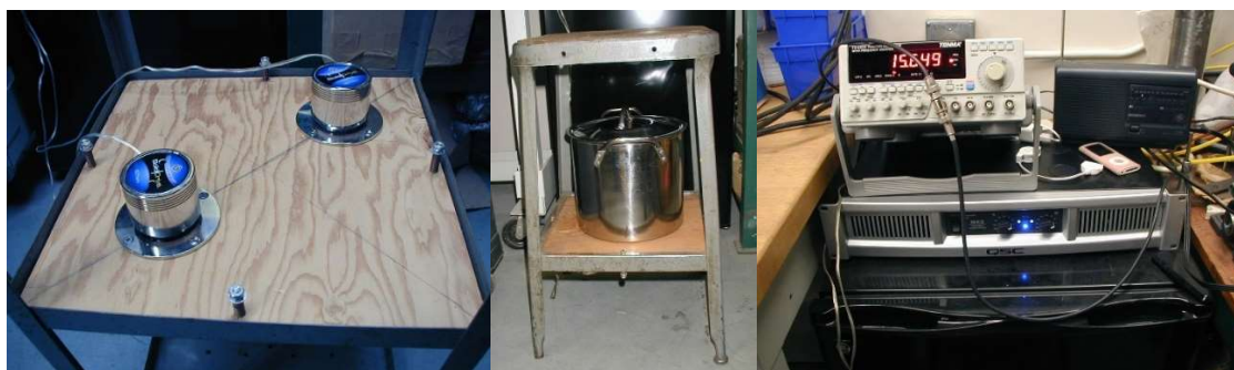
Figure 57: Mold belt soaking in DCM on Acoustically driven platform.
