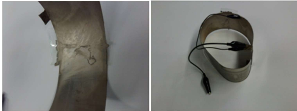
Figure 48: Flaws from the conductive silver paint.
