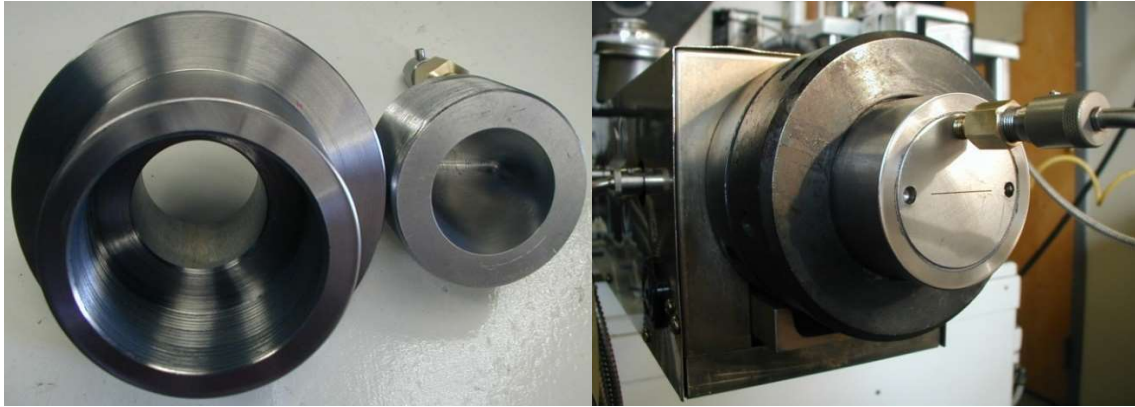
Figure 6: Compact design ribbon die made using EDM.
