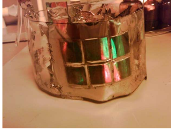
Figure 55: The nickel separated from the mandrel under plating tensile stress.
