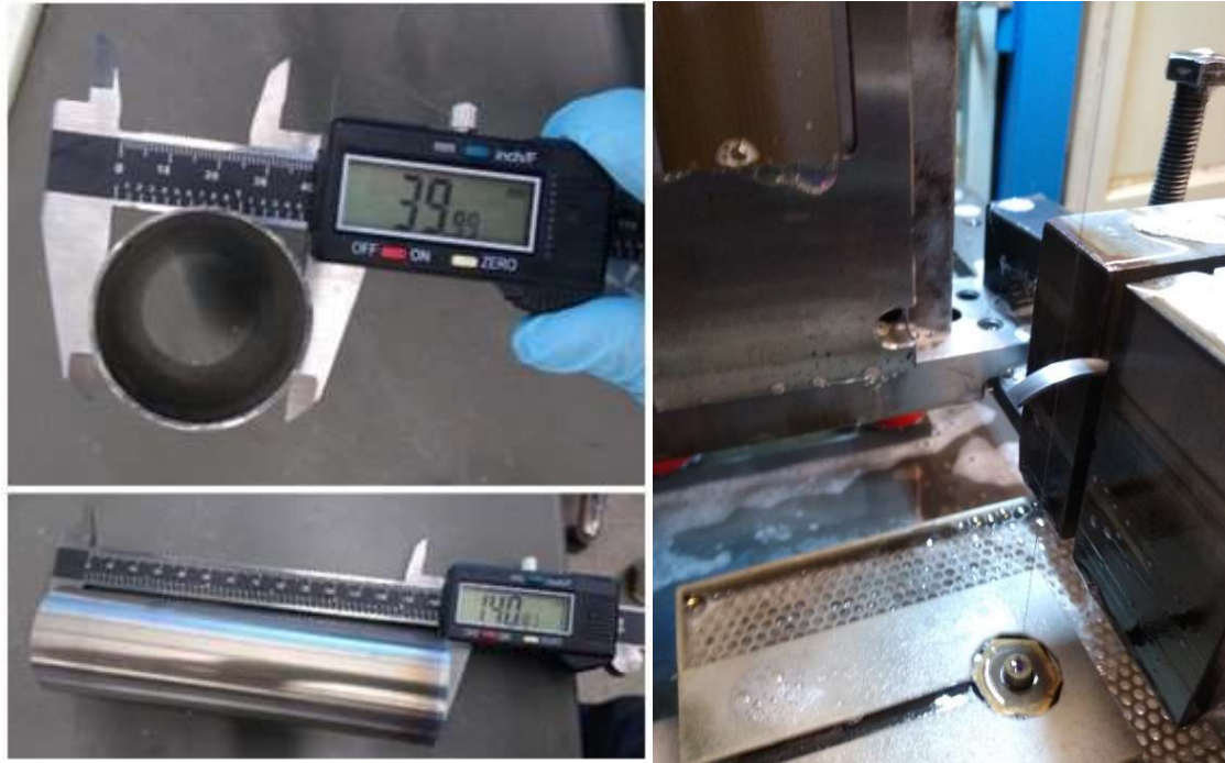
Figure 60: A 5 mm wide ring section of the MG cylinder, in the EDM to cut 5 mm sections.
