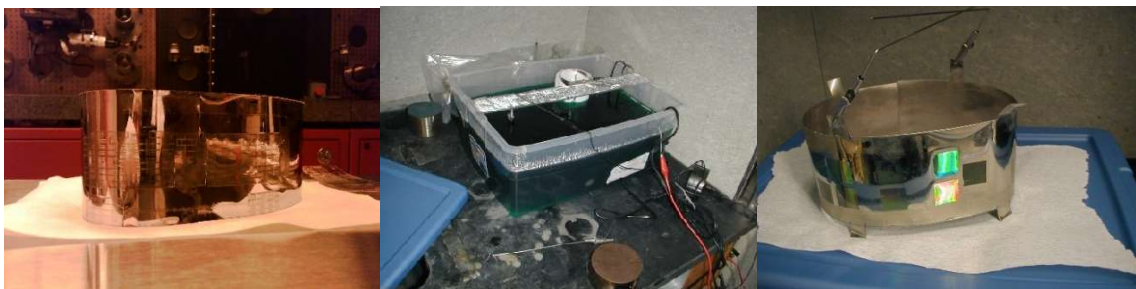
Figure 25: PET with seed Ni, plating bath and 200 \mu\text{m} thick nickel belt.
