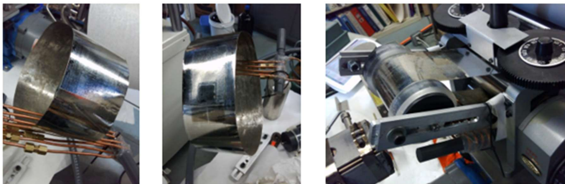
Figure 51: Mold ribbon belt being installed.
