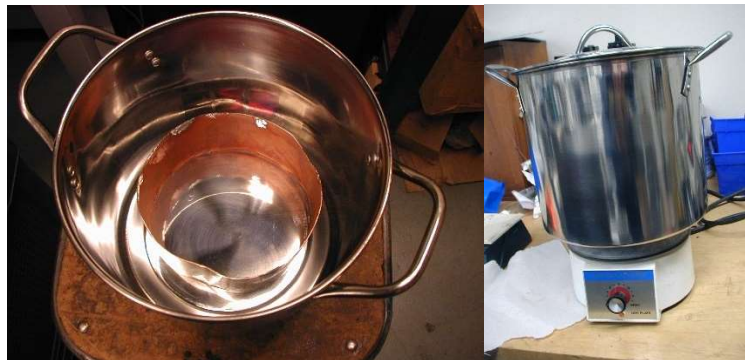
Figure 56: NOA 81 contaminated belt mold soaking in DCM and heated.
