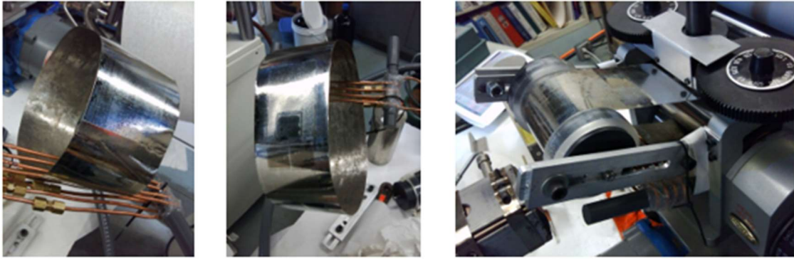
Figure 26: Ribbon belt mold being installed.
