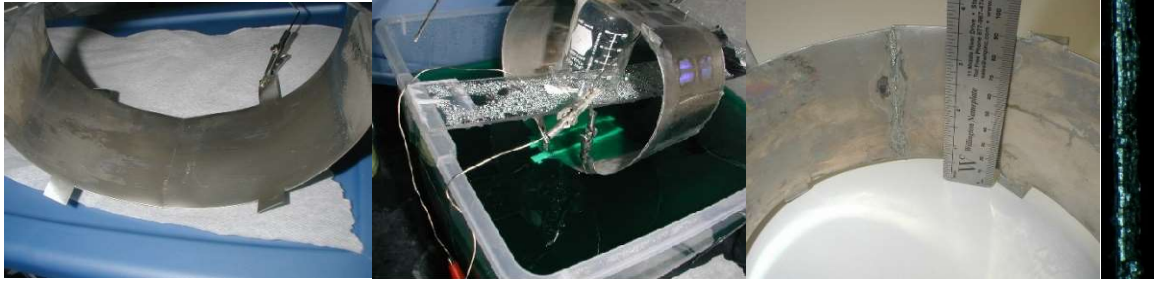
Figure 52: Weak seam, plating over seam, stronger seam, view through microscope.
