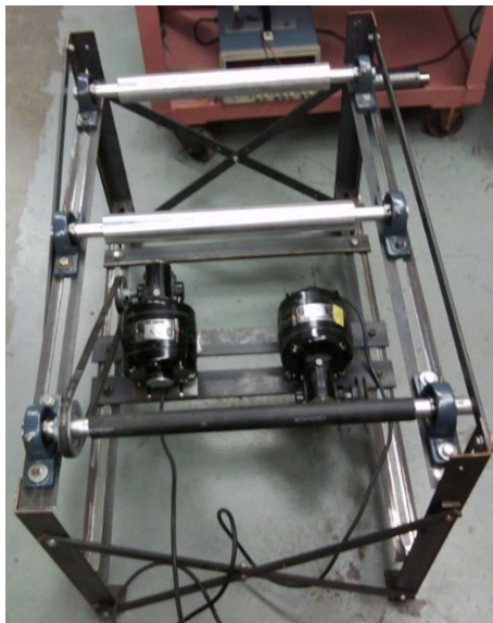
Figure 29: Cooling rollers and winder
