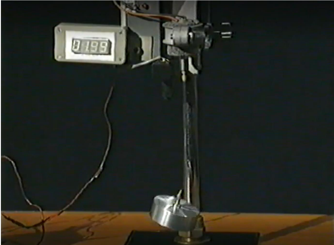
Figure 3.1. Experimental thin wire rotor undergoing gyroscopic motion [17].
