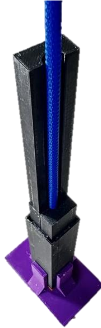
Figure 17. Complete Silicone Artery Molding Jig.
