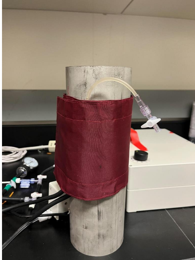
Figure 31. Steel Cylinder and Medical IV Bag Used for Device Validation.
