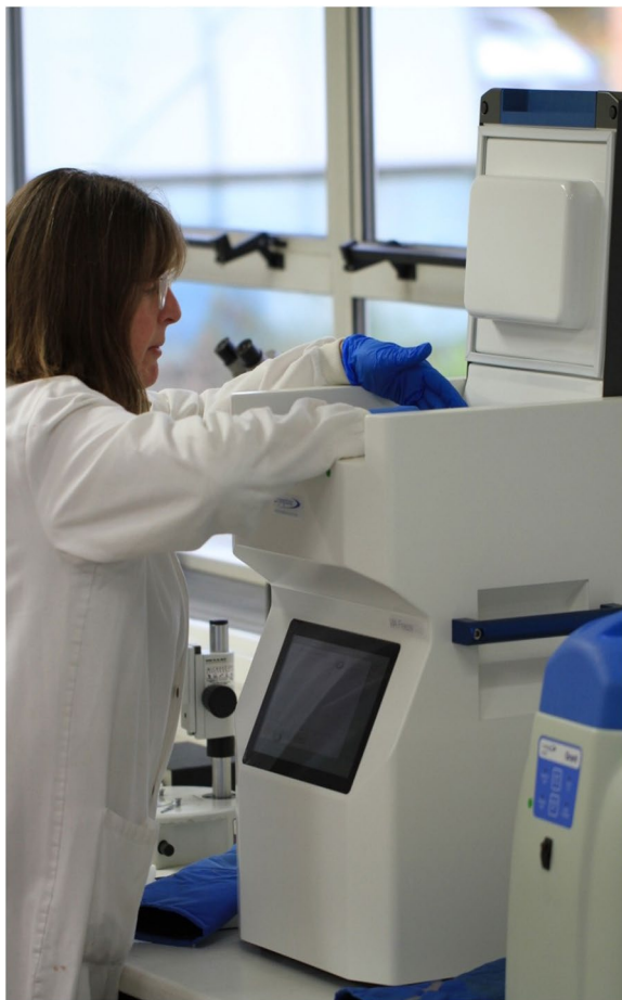
Fig. 4 Via Freeze™ duo Stirling cycle cooler and operator
