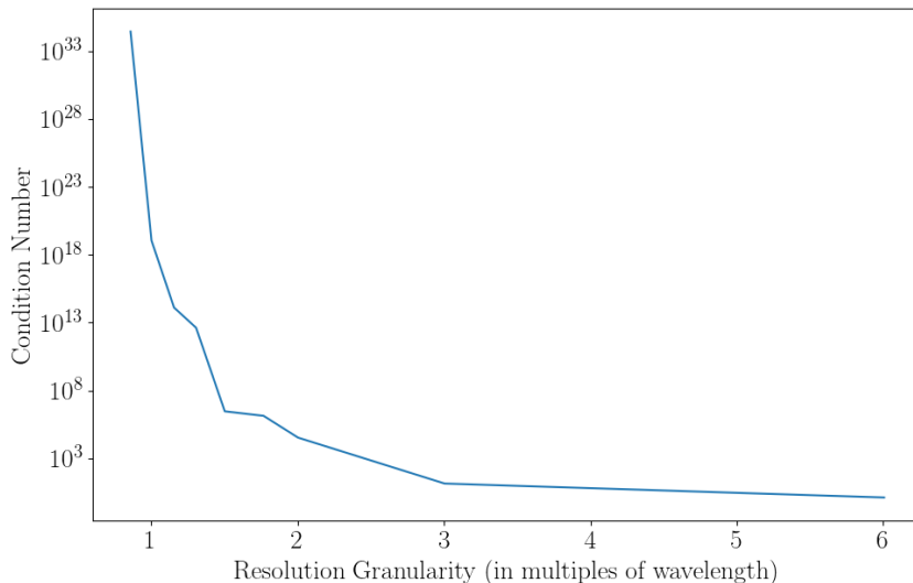
Impact of Resolution on the Condition Number of a SAR Observation Matrix
