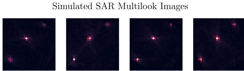
Figure 5.5: Figures displaying simulated backprojected images of the same scene imaged using differing flight paths.
