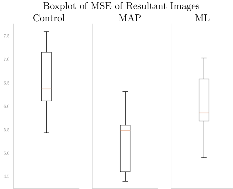
Figure 5.7: Boxplots showing the MSE of the obtained images using the MAP and ML approaches. The control plot represents the average MSE of the sum of the original set of images.
