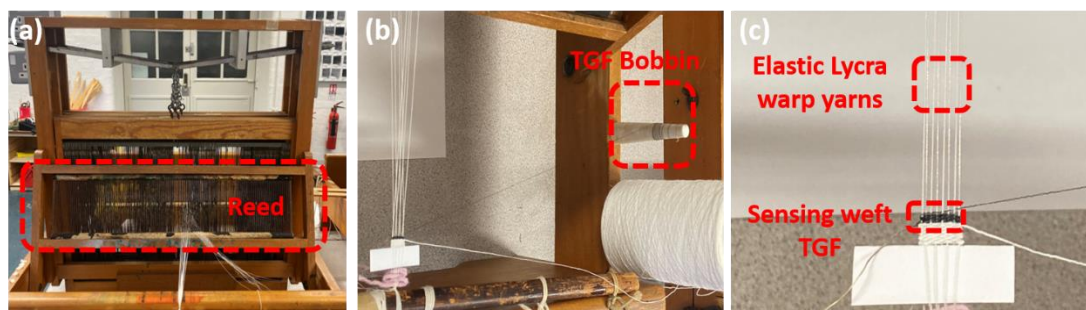
Figure S5-5. Fabrication of the BWWAJ strain sensor. a) hand weaving loom. b) hand weaving process with TGF bobbin. c) plain weave sensor structures constructed by weft TGF and elastic Lycra warp yarns.
