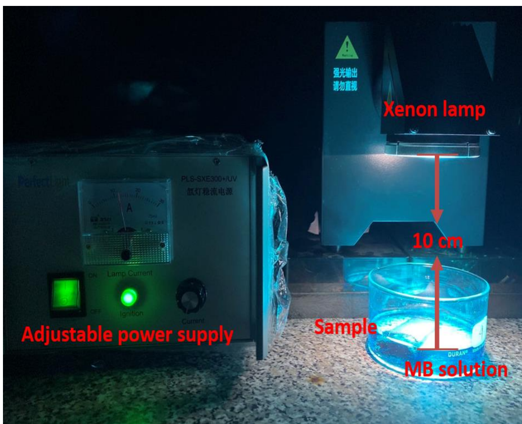
Figure S3-5. Illustration of photocatalytic degradation measurements.
