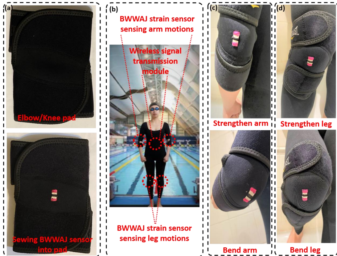
Figure S5-17. Photographs of integrated wearable BWWAJ strain sensors on the arthrosis of athlete. a) Sewing BWWAJ strain sensors onto elbow and knee pads. b)
