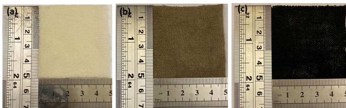
Figure S3-1. Images of 5×5 cm wool fabric before and after treatment. a) Pristine 5×5 cm wool fabric. b) FF-20%GO after pad-dyeing process. c) FF-20%rGO after L-ascorbic acid (L-AA) reduction.
