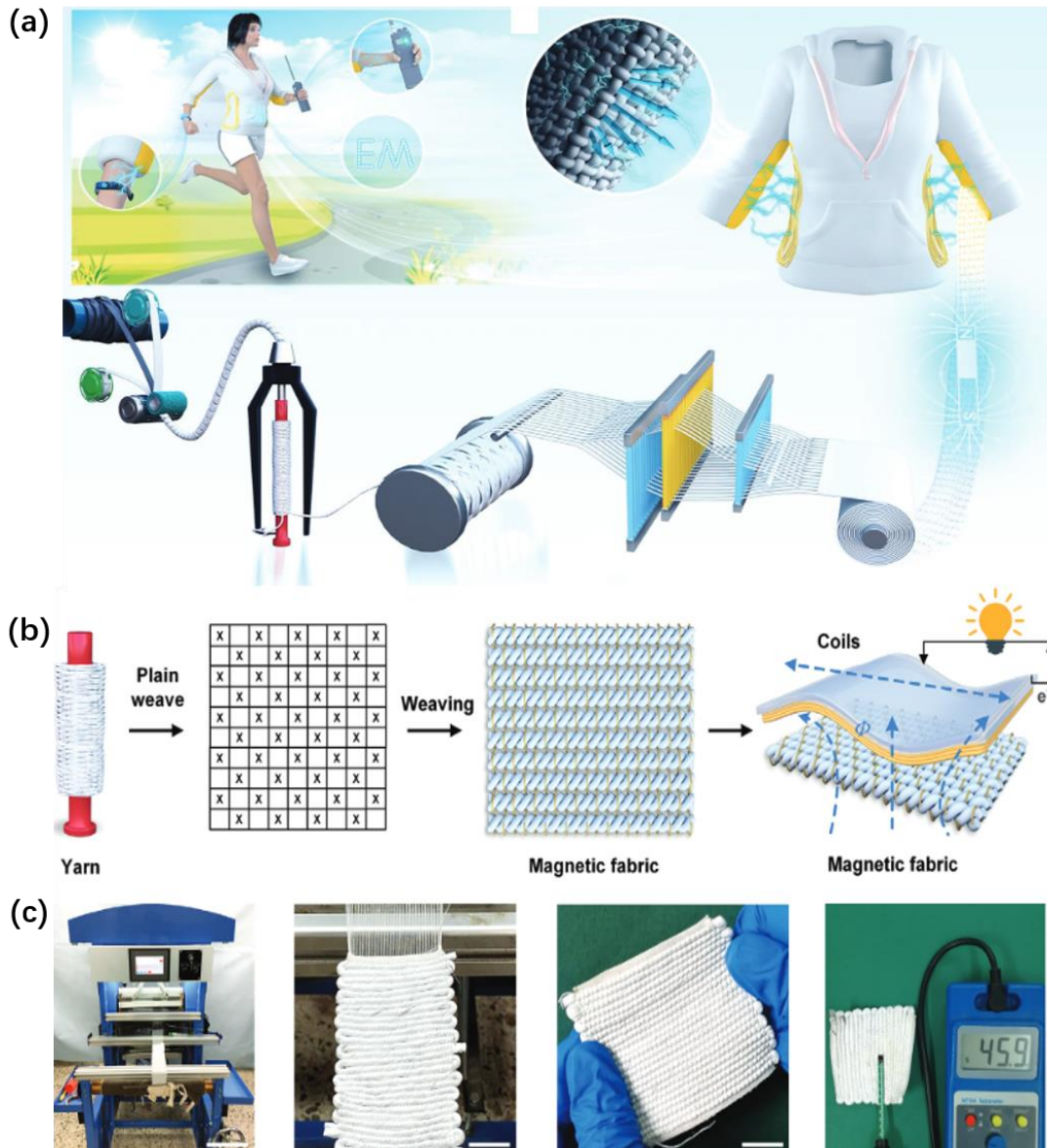
Figure 2-15. A plain-woven magnetic fabric for energy harvesting. 6 a) The preparation of a plain-woven magnetic fabric and schematic illustration of a magnetoelectrical clothing. b) Plain-woven structure of the magnetic fabric. c) Images of weaving loom and magnetic fabrics.
