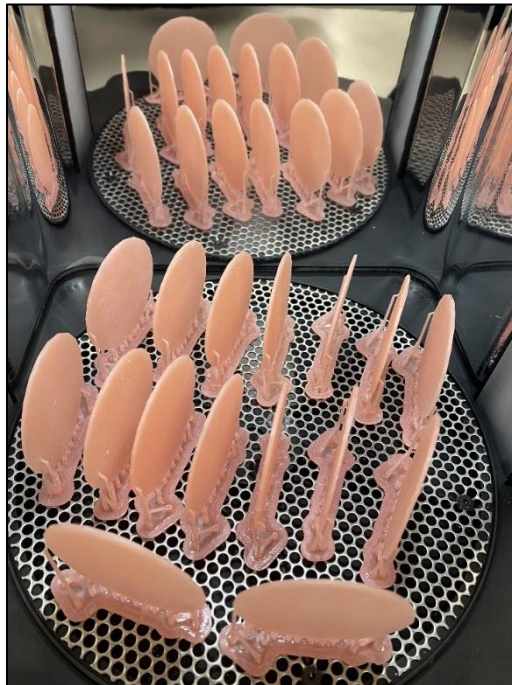
Figure 3.5. Specimen were placed in a UV light box for final polymerisation.
