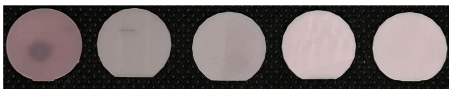
Figure 0.8. Colours of specimens of 3D-printed/ \text{TiO}_2 NPs composite material with concentration of 0.0, 0.10, 0.25, 0.50, and 0.75 wt.% from left to right
