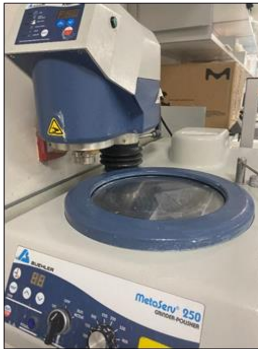
Figure 3.6. Polishing lapping machine
