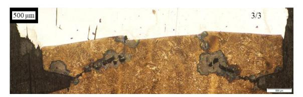
Picture V-n: cold cracks in the heat-affected zone (sample MND6, cutting planes 1/3 and 3/3)
