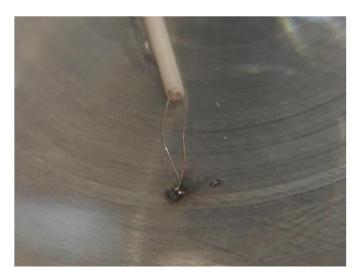
**Picture IV-d:** spot-welded micro-thermocouples on a sample representing the upper surface of the Jominy specimen (PASEPMARTY1 sample)
