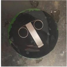
**Picture V-k:** sample machining on a lathe to expose a longitudinal cutting plane (the surrounding cylinder has been removed in this case)
