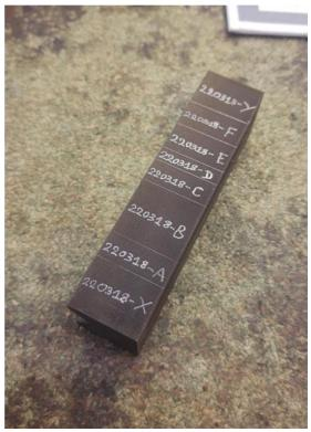
Picture V-f: extraction by electrical discharge machining of the weldment and sample reference engraving prior to the cutting in "slice" samples (220314-TEK1-WH-SS & 220318-TEK2-WH-SS mock-ups)
