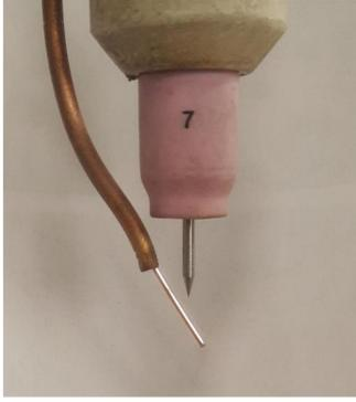
**Picture IV-h:** tungsten inert gas welding torch configuration and example of dummy mock-up used to make sure the installation was functioning properly
