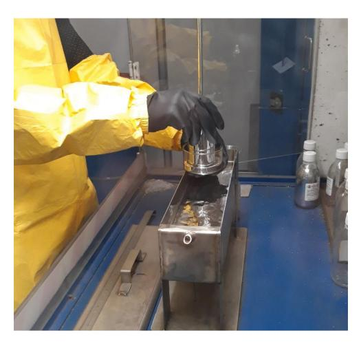
Picture III-b: analysis of an ISO 3690 sample using metallic mercury (source : the IS)
