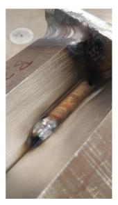
**Picture IV-i:** one of the y-slot dummy mock-ups used to make sure the installation and the weld program were functioning properly
