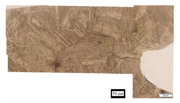
**Picture V-o:** small cold crack in the heat-affected zone (sample MND7, cutting plane 2/3)
