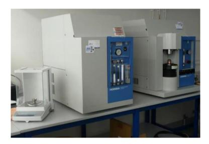
**Picture VI-h:** Jobin Yvon Horiba EMGA-621W hydrogen analyser (scale, furnace, and hydrogen detector)
