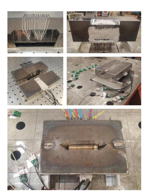
**Picture IV-j:** the thermocouple-instrumented mock-up before and after assembly, and after the welding run completion (220406-TEK1-WH-INC-TC specimen)
