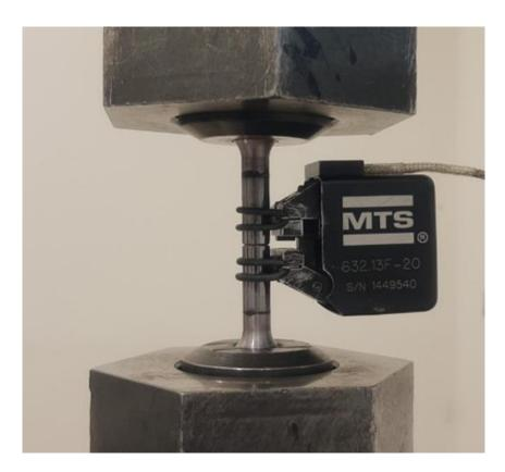
**Picture VI-i:** positioning of a notched specimen on the testing machine
