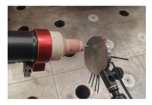
**Picture IV-e:** alignment of the arc-welding torch electrode and the pyrometer beam spot with the micro-thermocouple (pyrometer beam spot represented by the laser targeting light feature – PASEPMARTY1 sample)
