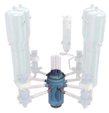
**Figure I-b:** focused view of a nuclear steam supply system (group **C**) highlighting the reactor pressure vessel (adapted from [19])
