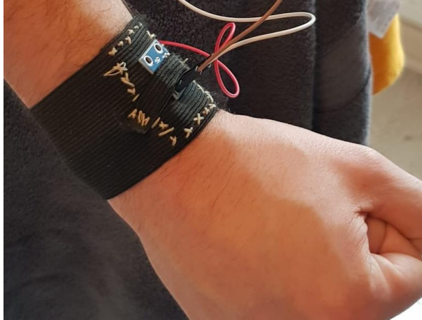
Figure 3-55. Wrist Mounted Accelerometer in position 3A
