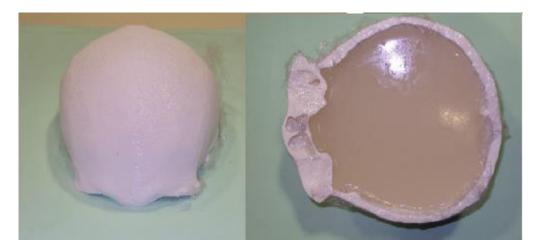
Figure 53: Menikou et al. head phantom compatible with MRI [259].
