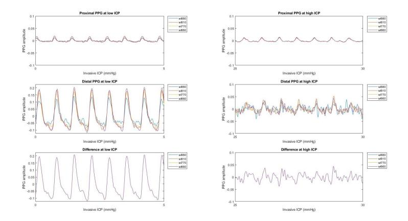
Figure 131: Zoom-in views of a 10 second window of the normalised PPG signals at the extreme values (5 mmHg and 30 mmHg) from both proximal and distal detectors of one replicate, including the difference between the detector's signals
