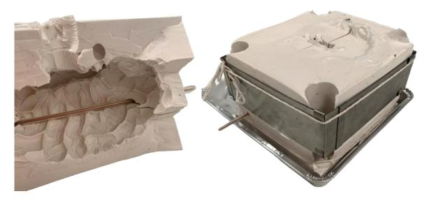
Figure 70: Brain mould with the middle cerebral artery, ready to receive the brain silicone mix.
