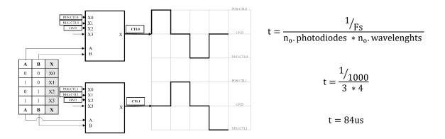
Figure 113: Multiplexing circuit
