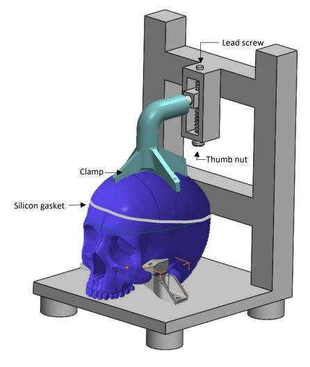
Compression system to seal the skull Figure 67: Final seal, compression system
