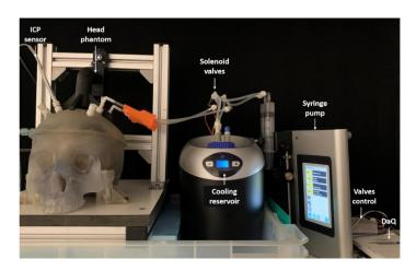
Figure 103: Phantom CSF circulatory system
