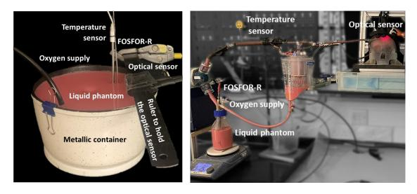
Figure 137: Phantom set up for non-invasive oxygenation measurements
