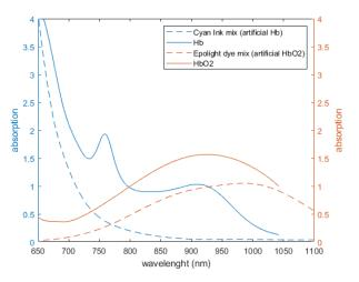
Absorption spectra of the mixtures (Cyan ink solution: artificial Hb, Epolight solution: artificial HbO2) compared to haemoglobin's spectra (scaled x5000).
