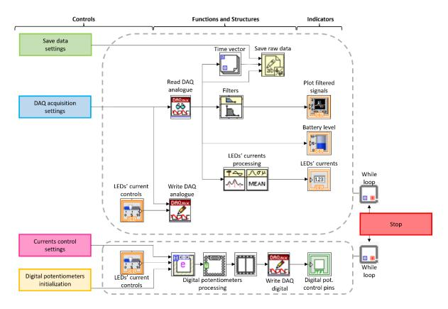
Figure 118: LabVIEW summarized Block Diagram for the TBI sensor
