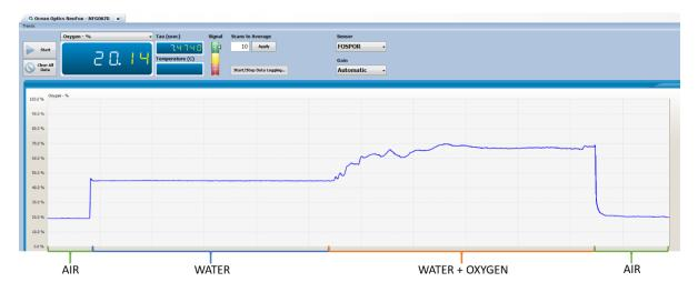
A. Response of the FOSPOR-R probe to diffused oxygen into the water.
