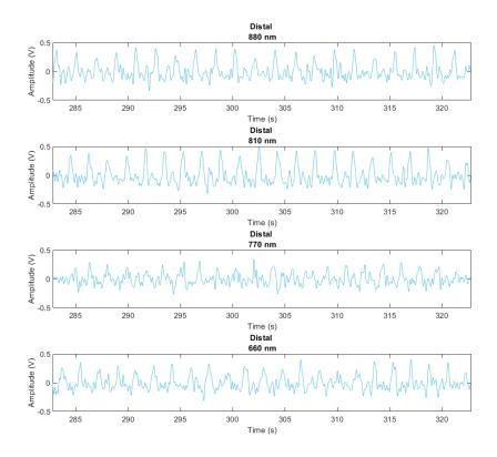
Figure 143: Pulsatile signals acquired from the head phantom using the liquid phantom fluid as blood
