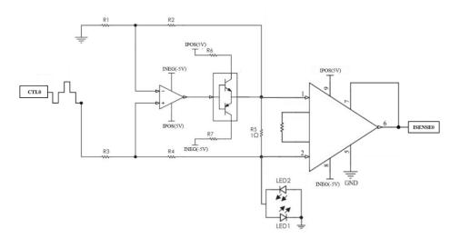
Figure 114: Current source schematic design
