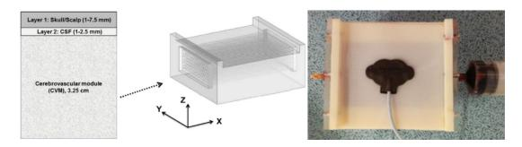
Figure 55: Afshari et al. head phantom for standardized testing of clinical NIRS oximeters [235].
