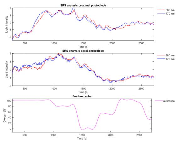
Figure 142: Normalized optical signals at 770 nm and 880 nm in comparison with the FOSFOR-R probe measurement, acquired from the head phantom using the liquid phantom fluid as blood
