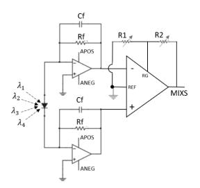
Figure 115: Differential transimpedance amplifier schematic design
