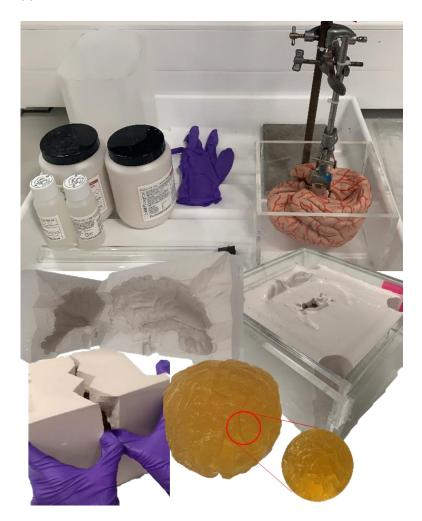
Figure 69: Brain mould manufacture
