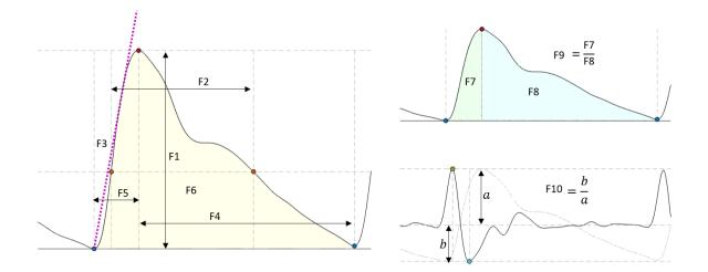
Figure 128: Features extracted from the optical signals
