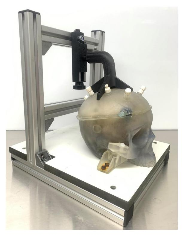
Figure 93: Final seal with compression structure
