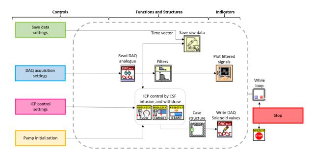
Figure 86: LabVIEW summarized Block Diagram for the phantom
