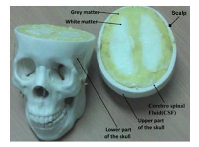
Figure 52: Mohammed et al. head phantom for microwave-based imaging [258].
