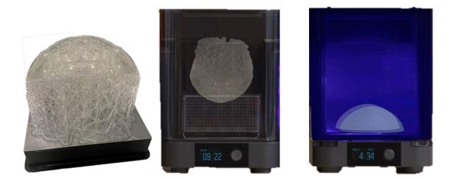
Figure 60: Formlabs port-curing process applied to the calvaria
