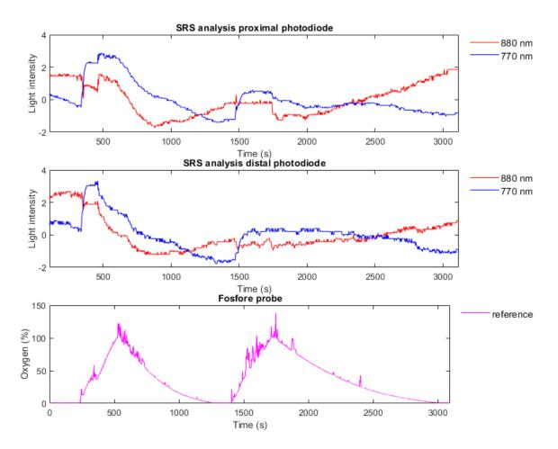
Figure 139: Normalized optical signals at 770 nm and 880 nm in comparison with the FOSFOR-R probe measurement
