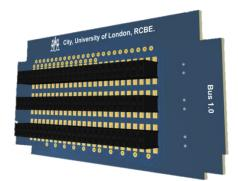
Figure 110: Bus connector 3D model
