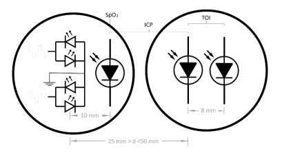
Figure 106: Probe configuration of the optical components
