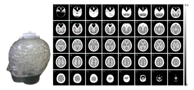
Figure 50: Iida et al. head phantom to evaluate PET/SPECT image quality [230].
