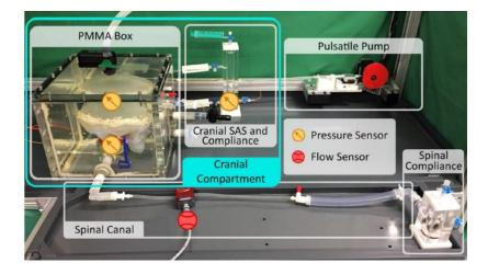
Figure 56:Benninghaus et al. phantom of the CSF system [240].
