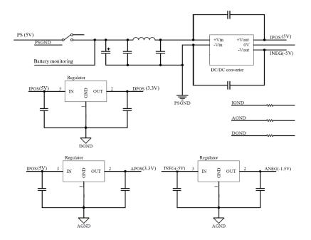
Figure 111:Power supply schematic design
