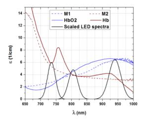
Extinction spectra of the dye mixtures (M1: HbO2 mixture, M2: Hb mixture) compared to haemoglobin's spectra. Figure copied from Akl's study [271].
