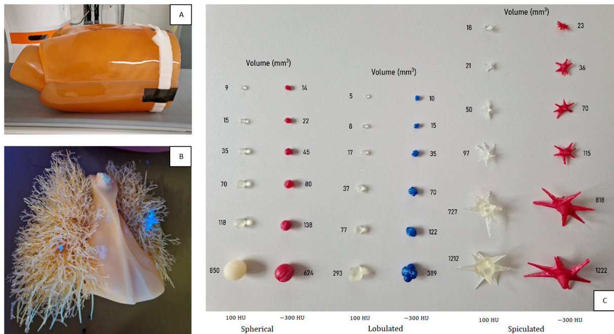
Figure 1. Overview of the phantom setup. (A) Anthropomorphic thorax phantom with tissue-equivalent chest plates, (B) 2 UV-reflective nodules inserted in the lungs, and (C) an overview of the 36 artificial nodules of different sizes, shapes, and densities. CT values of the subsolid (red and blue) and solid (translucent white) nodules were -330 \pm 50 HU and 100 \pm 30 HU, respectively. Volumes ranged from 5 to 1222 mm 3 .
