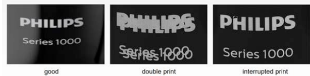
Fig. 1. Examples for the three classes present in the dataset provided by Philips Consumer Lifestyle BV . The dataset is imbalanced. Most images correspond to non-defective pieces (good print), while the defective prints (double or interrupted prints) introduce different levels of imbalance.
