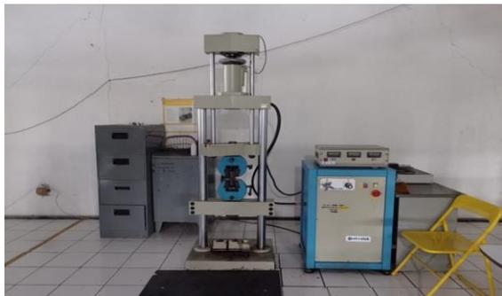
**Gambar 3.** *Universal Testing Machine (UTM) type TN20MD*
