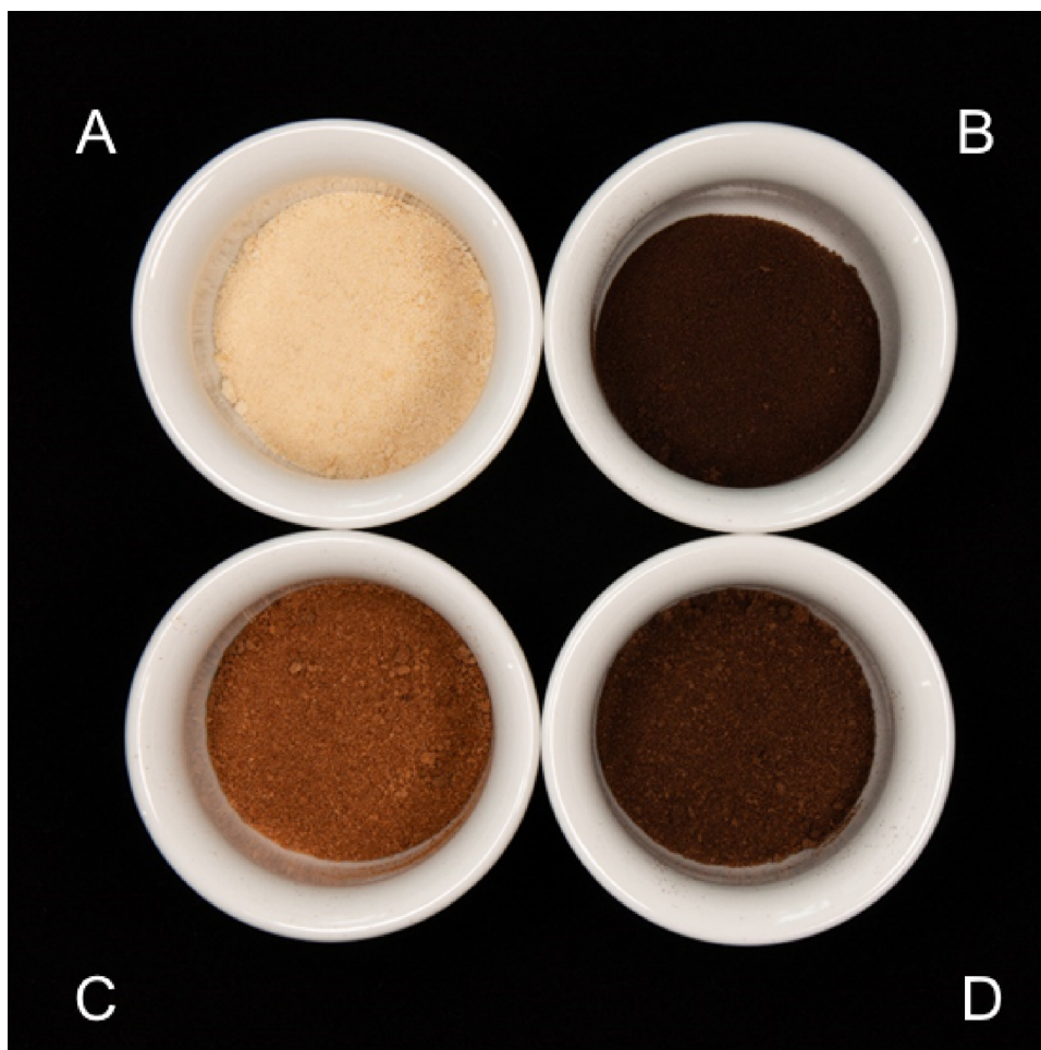
Figure 1. Coffee cell samples: (A) Unroasted, lyophilized coffee cells ( L^* = 48.8 ); (B) roast 1 ( L^* = 31.0 ); (C) roast 2 ( L^* = 36.0 ); (D) roast 3 ( L^* = 32.0 ) (roasting conditions described in section 2.2). L^* = lightness value (dark–light, 0–100) according to the color spacer defined by the International Commission of Illumination (CIE).
