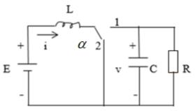
Fig. 1. A DC-DC boost power converter: the inductor L, load resistor R, capacitor C, input voltage E, switch position $\alpha$ , inductor current i and capacitor voltage v
