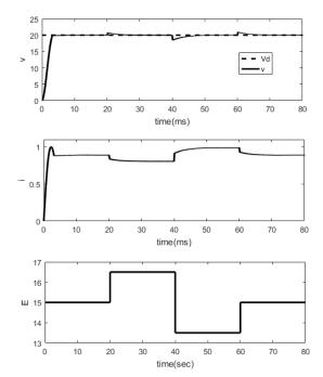
Fig. 9. The results of the PBC when E changes: the capacitor voltage v and inductor current i and input voltage E
