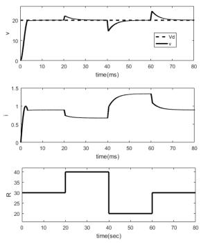
Fig. 7. The results of the SMC when R changes: the capacitor voltage v and inductor current i and load resistor R  $\,$
