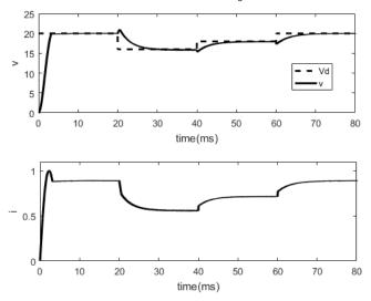
Fig. 3. The results of the PBC when  $V_{\text{d}}$  changes: the capacitor voltage v and inductor current i
