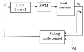
Fig. 2. The structure of sliding mode control for a DC-DC boost power converter: the inductor current  $x_1$ , the capacitor  $x_2$ , control input  $\mu$  and desired voltage  $V_d$
