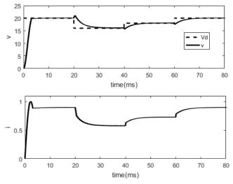
Fig. 4. The results of the SMC when  $V_{\text{d}}$  changes: the capacitor voltage v and inductor current i
