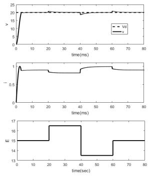
Fig. 11. The results of the PBC-SMC when E changes: the capacitor voltage v and inductor current i and input voltage E  $\,$
