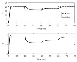
Fig. 5. The results of the PBC-SMC when  $V_{\rm d}$  changes: the capacitor voltage v and inductor current i
