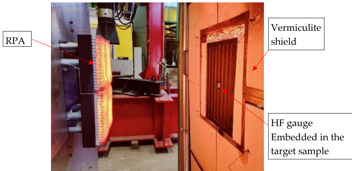
Figure 3 An example of the set up used to measure the heat feedback from the target samples to the RPA. The vermiculite shield can be seen in the picture too.
