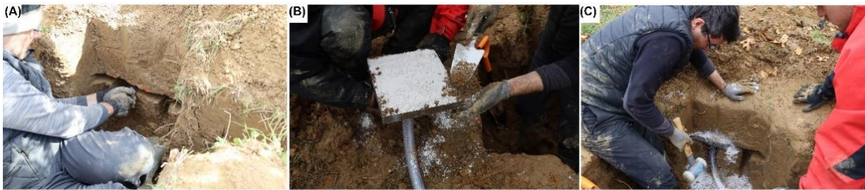
Figure 3. Process of installation of passive wick lysimeters: (A) precision cutting, (B) lysimeter assembly and application of crushed soil and quartz flour, and (C) positioning the lysimeter with a hammer at the SUPREHILL Critical Zone Observatory (CZO).
