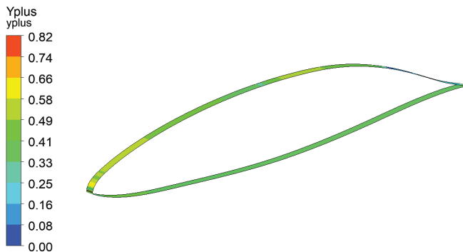
Figure 3: Dimensionless y^+ values on the hydrofoil surface.
