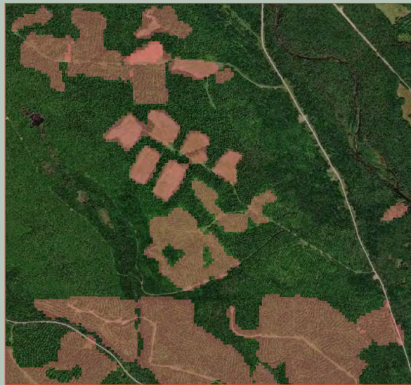
IGS forest change detection sample, 30 m resolution, superimposed over high resolution digital photography.
