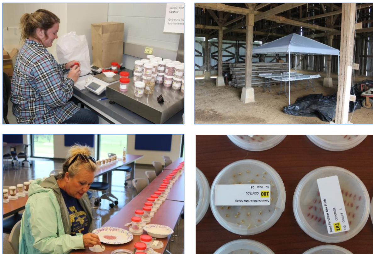
Figure 1. Seed and fertilizer were weighed out and placed into 120 ml cups (top right) and uncapped cups were placed under a canopy in a tobacco barn (top left) for 1 to 28 days. Cups were transported back to the lab at specified exposure intervals and 50 random seeds were extracted (bottom left) and placed into a petri dish for germination (bottom right).
