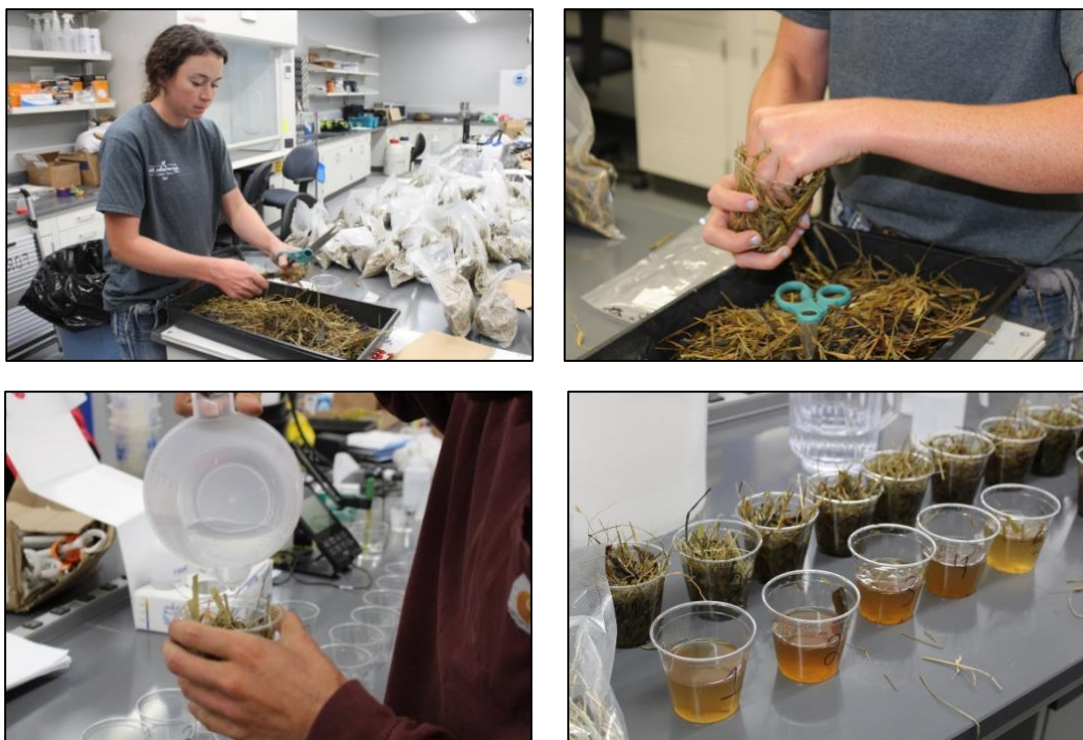
Figure 2. After six weeks of fermentation, silos were opened (top left) and a sample from each was submerged in distilled water for pH determination (top left and bottom). The remaining sample was dried and ground for nutritive value determination.
