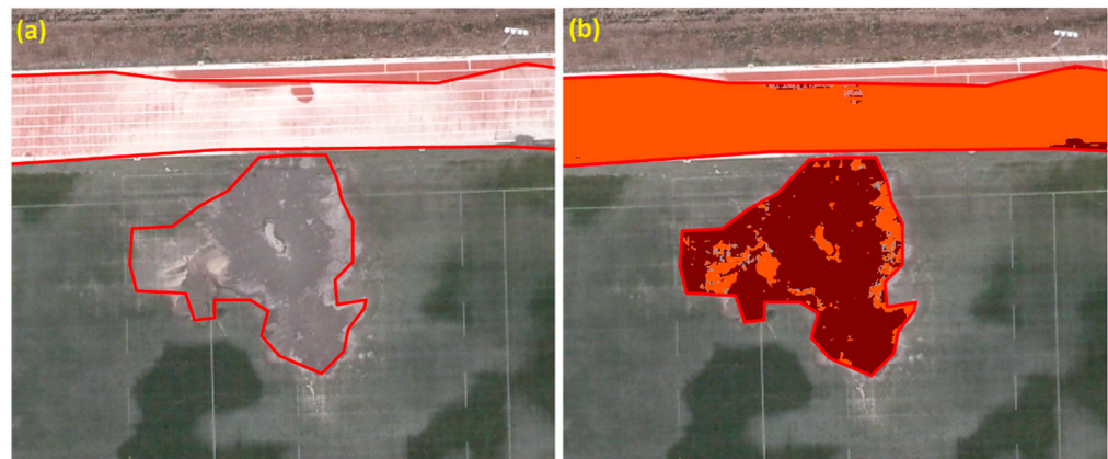
Figure 6. (a) An example of the liquefaction ejecta polygons drawn by Sanon et al. (2022) [43]. (b) Fuzzy C-Means clustering results for the example image tile with dark and light liquefaction. The dark red and orange colors are indicators of dark and light liquefaction, respectively. Uncertain pixels are removed from liquefaction training data based on their low probability of belonging to any of the dark or light liquefaction classes.
