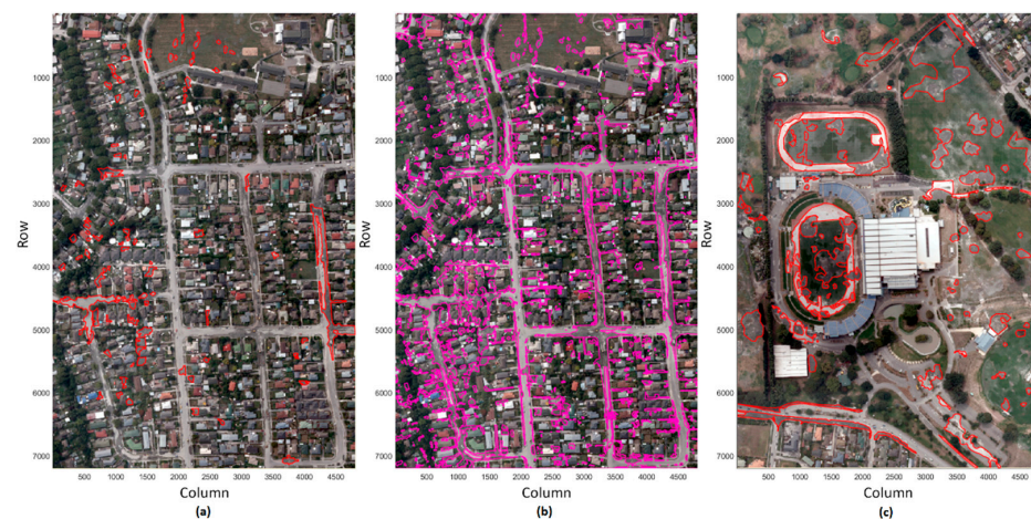
Figure 3. (a) The image tile used for model development and evaluation with Sanon et al. (2022) [43] liquefaction polygons (in red) overlaid. (b) The image tile with a complete label (in magenta) was created for model validation in this study. (c) The image tile used for model application with Sanon et al. (2022) [43] liquefaction polygons (in red) overlaid. Row and column are indicators of pixel number in each axis of the image shown in the figure.
