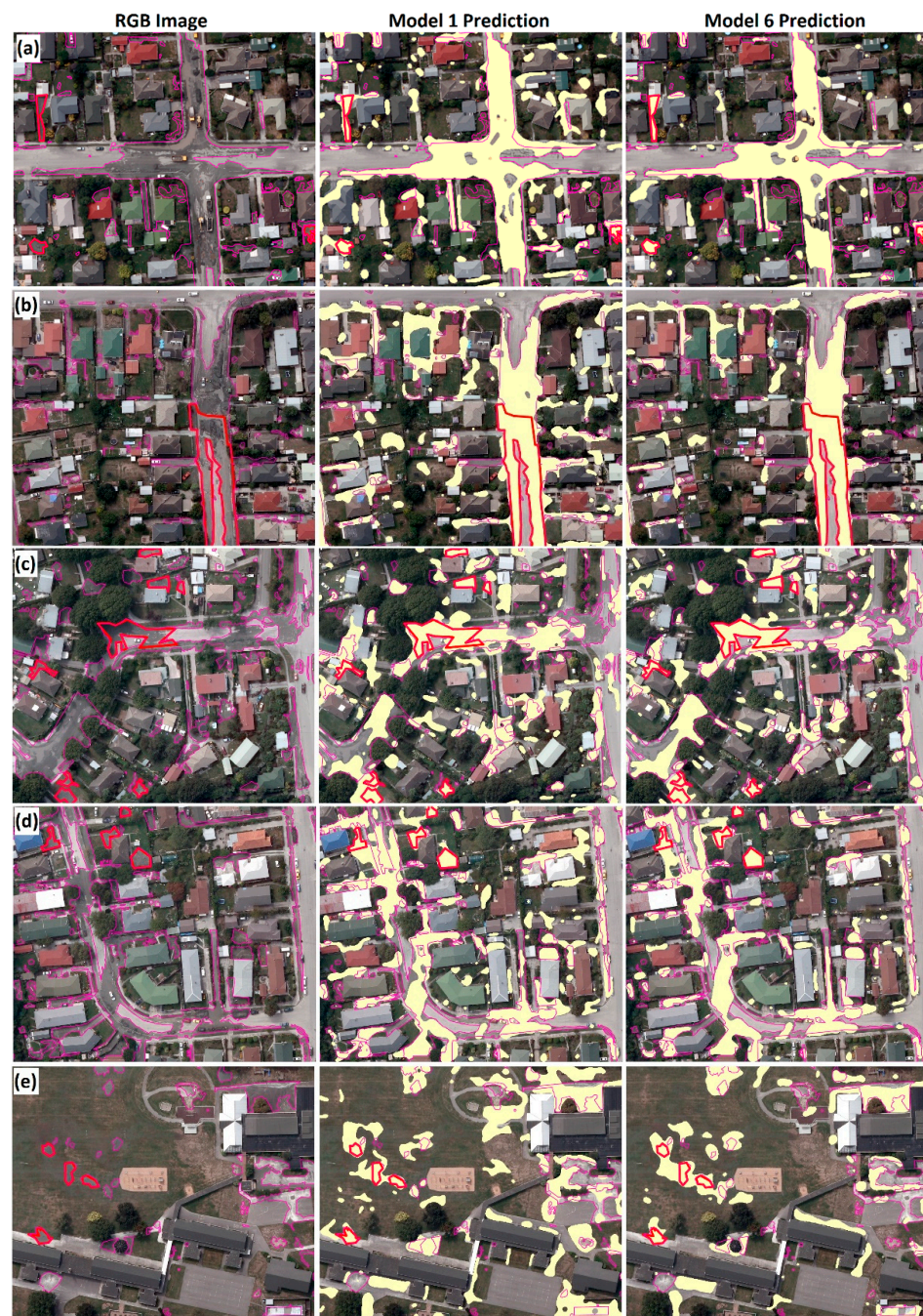
Figure 16. Binary classification results of Model 1 (RGB-based model in the middle column) and Model 6 (preferred model in the right column) with Sanon et al. (2022) [43] liquefaction polygons (in thick red) and validation labels (in magenta) overlaying the model prediction (in yellow). (a–e) Example regions in the model development tile visualized for evaluation of the predictions.
