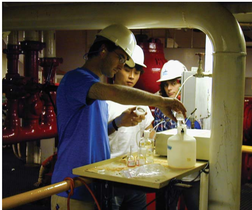
Figure 1. Subsampling (left) and adding tracer to drilling fluids (right).
