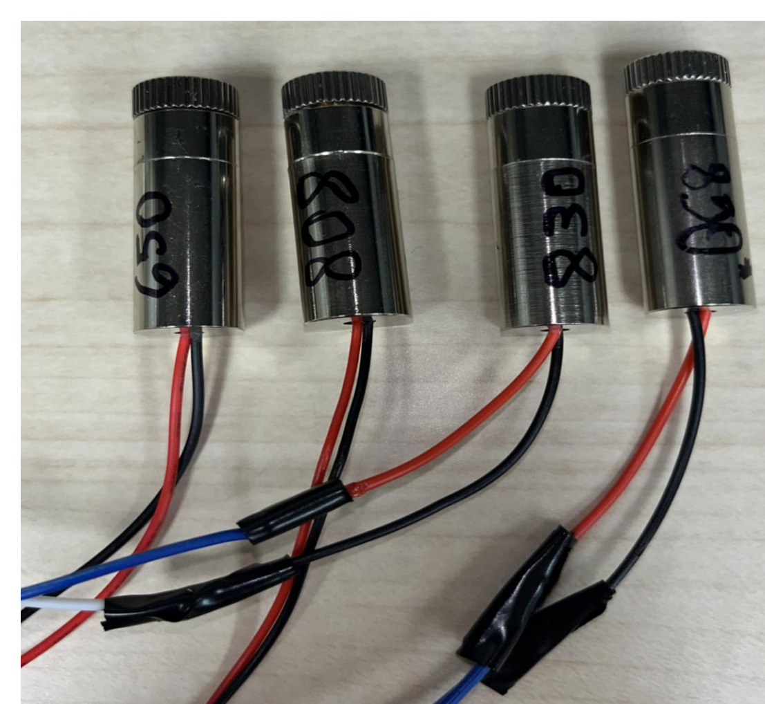
Image shows the (From left to right) 650nm, 808nm, 830nm, & 850nm lasers.
