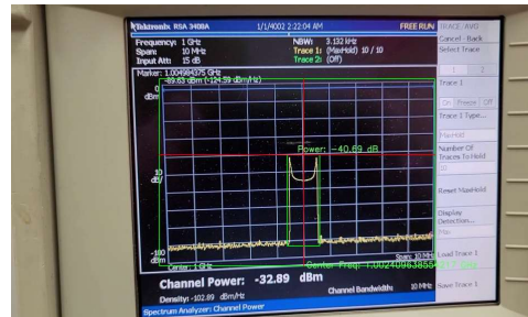
Figure 2. Carrier Signal with Single Sideband Modulation
