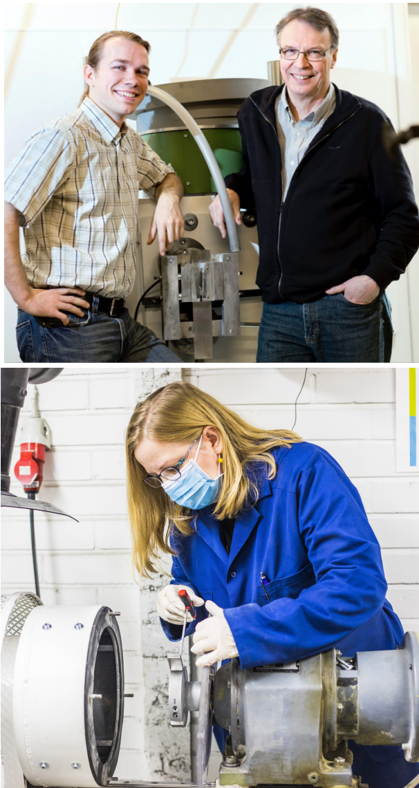
Figure 9.2.2 (a) The doctoral student Juuso Terva (left) designed and built a dual pivoted jaw crusher for wear studies at Tampere Wear Center supervised by professor Veli-Tapani Kuokkala (right) in 2015. (b) Dr Kati Valtonen attaching samples to the impeller-tumbler device. Photos: TAU/archive
