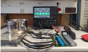
Fig. 13. Experimental test-bench including the IH coils, the pot, the power electronics prototype and the oscilloscope to capture the converter waveforms.
