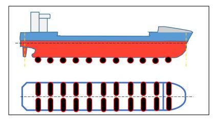
Figure 3. Two-line arrangement.
