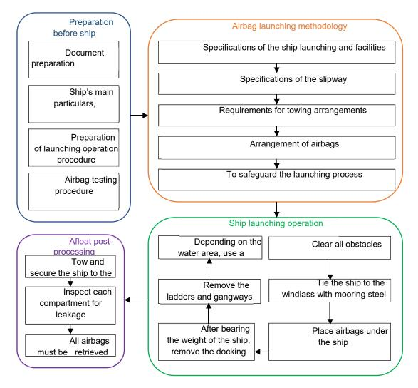
Figure 5. Ship launching operation flow.
