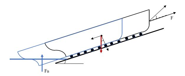
Figure 4. Force components of a ship.
