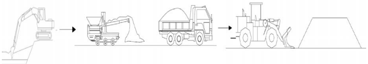
Fig. 2-6 Two stages construction method using lightly lime/cement treated clayey soils (Hino et al., 2008)
