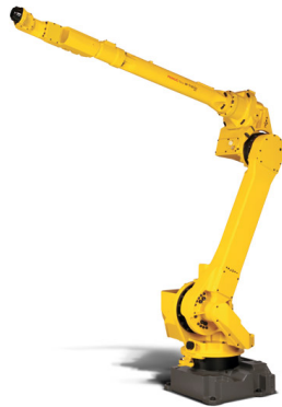
Figure 2. The FANUC M-710iC/12L robot arm which is planned to be used to control the glider [3].
