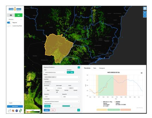
Figure 16 - The Brazilian instance of the GLAM System, showing a plot for soybean in Mato Grosso do Sul for NDVI from Terra (MOD09Q1) 8-day 250m – both the current season (~September 2020 – Present (Dec 2020), and the 10-year median observed soybean NDVI. The plotting interface allows for the overplot of crop calendar information along other utilities to provide context for the user.
