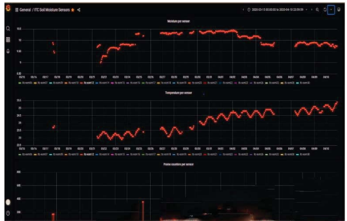
Fig. 6. IoT-WSN collected soil moisture and temperature data on Grafana web dashboard
