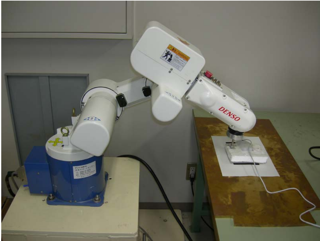
Figure 2.1: A robot arm is used to control movement of the optical mouse sensor.
