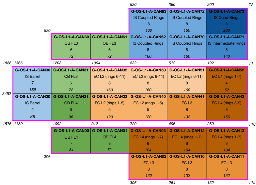
Figure C.1: Optobox distribution in the A-side sector 1 Optopanel (DFT a1-8). Each box represents an Optobox, its background colour is to distinguish the different layers. The Optobox ID is bold and the layer name is given below. The first number in each box is the amount of Optoboards and the italic number the amount of Twinax cables ending at that Optobox. The thicker, coloured border indicates the source of powering cavern.
