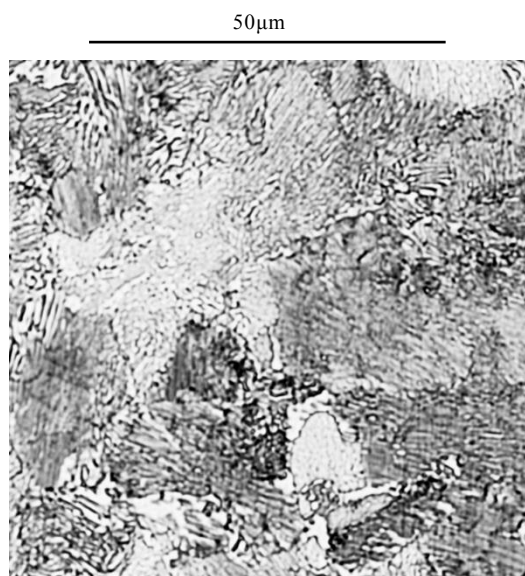
Partial magnification of Fig. 2-3 (e) (Normalized at 900°C)
