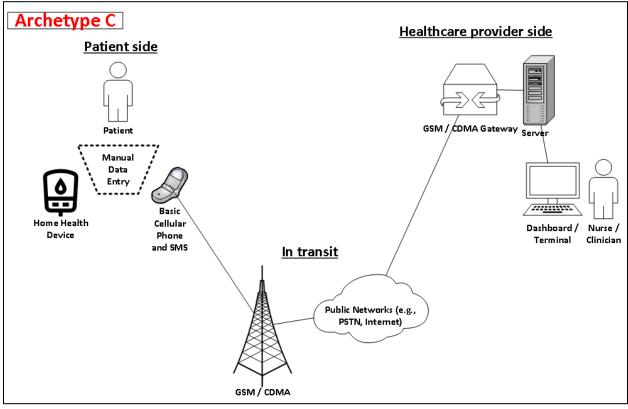
Figure 2.8. Archetype C. Telemedicine via basic cellular phone functionality.
