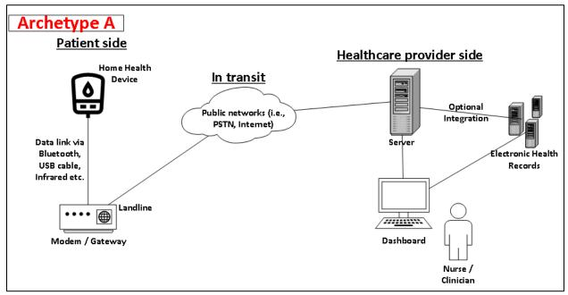
Figure 2.6. Archetype A. Telemedicine via connected health gateways with optional EHR integration.
