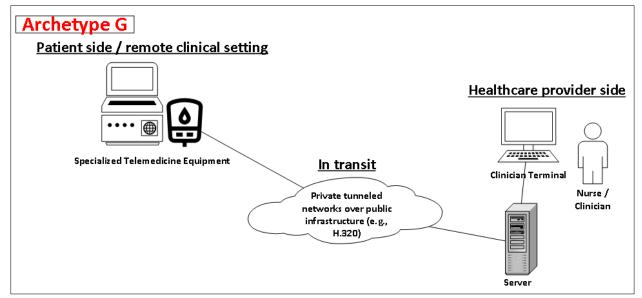
Figure 2.12. Archetype G. Telemedicine via specialized equipment with a provider-premises server.
