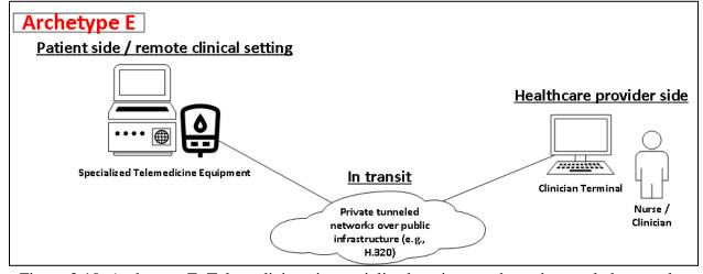
Figure 2.10. Archetype E. Telemedicine via specialized equipment through tunneled networks over public infrastructure.
