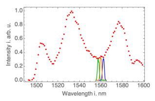
Figure 3: Shown is a graph with single measurements (green, yellow, blue) using the described setup using a slit and a collimator and the maxima of fits to all single measurements plotted with red dots reproducing the spectral shape.
