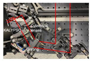
Figure 4: Shown is a photo of the spectrometer setup with an illustration of the two beam paths and the optical elements (grating, two cylindrical lenses and KALYPSO).
