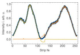
Figure 5: Shown are the intensities detected with KALYPSO plotted against the strip number. The measurement with two beam spots (thick blue line) is overlaid with two further measurements (yellow, orange) where one beam path was blocked.
