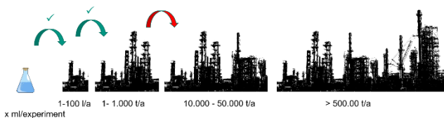
Figure 6: exemplaric scaling steps for chemical process ramp up
