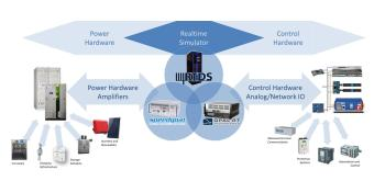
FIGURE 10. Concept of the Center for Applied System Simulations
