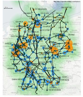
FIGURE 2. Transmission network model of Germany with generation/load and voltage heatmap.
