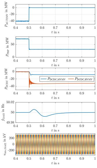
FIGURE 7. Example simulation for blocking station 2 and islanding
