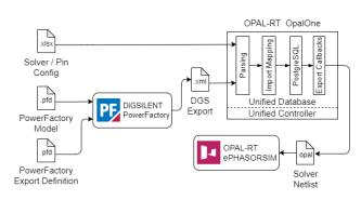
FIGURE 16. Model conversion from PowerFactory to ePHASORSIM using the Unified Database.
