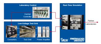
FIGURE 14. Concept of Co-Demonstration Platform at the Distribution Grid Laboratory at RWTH Aachen University
