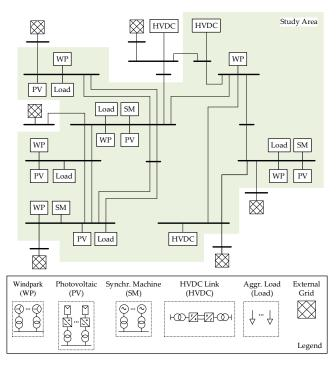
FIGURE 3. Schematic single line diagram of real-time model
