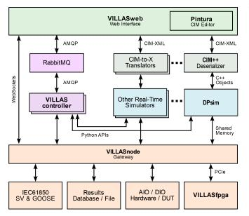
FIGURE 15. Architecture of the VILLASframework. Reprinted from [45]
