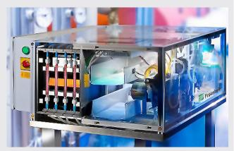
In the biological broadband sensor »AquaBioTox«, microorganisms are continuously flushed with drinking water. A camera with automatic image analysis detects changes that trigger an alarm signal.
