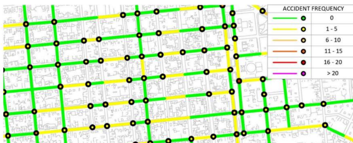
Figure 4. Example of a part of a crash frequency map for an urban city network (based on [58]).
