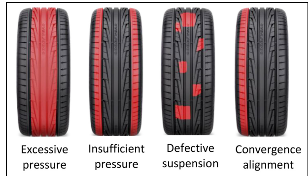
Figure 1. Typical wear states.
