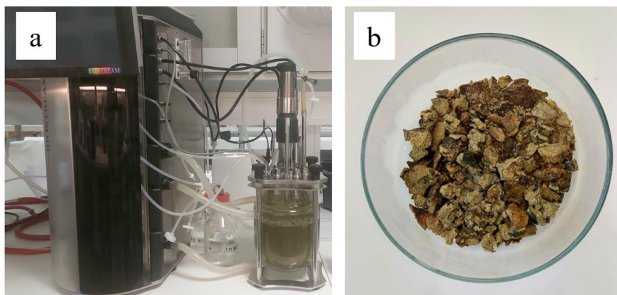
Figure 27 Fermentation setup with a 2 L bioreactor vessel (a) and an example of protein-enriched concentrate obtained after precipitation, centrifugation and oven drying (b).
