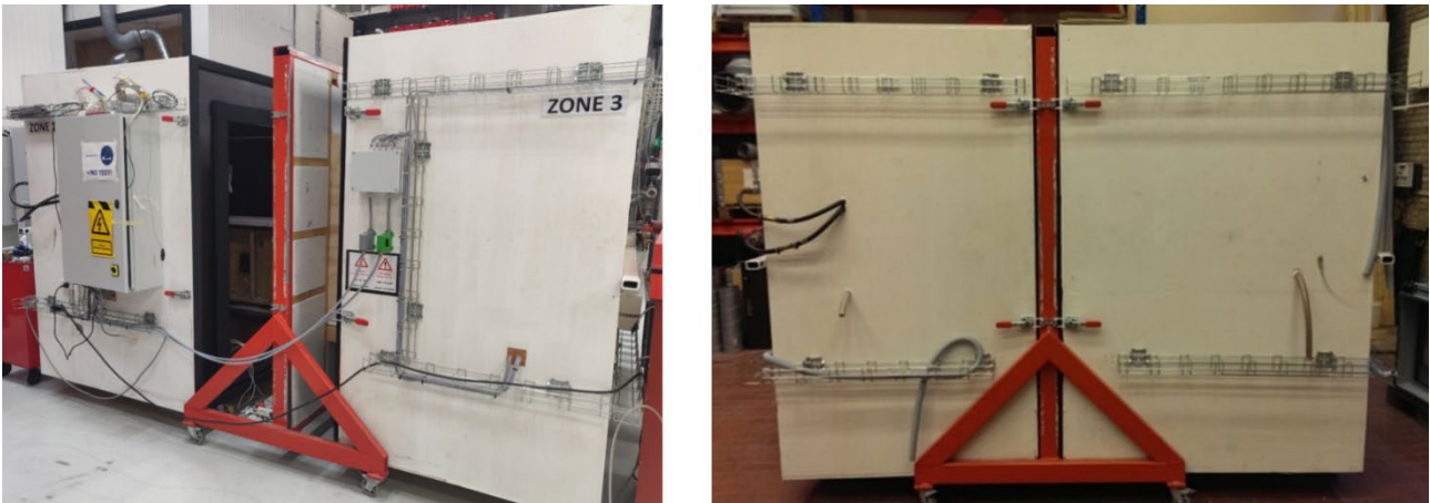
Figure 4: The Guarded Hot Box setup at Aalborg University, Department of the Built Environment.
