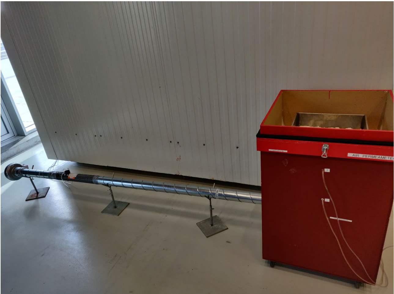
Figure 10: Air permeameter setup [10].
