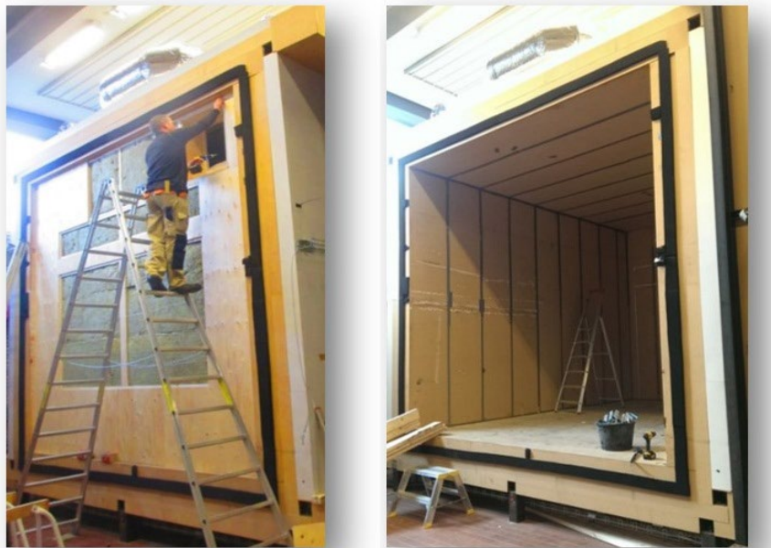
Figure 5: The Big Guarded Hot Box setup at Aalborg University, Department of the Built Environment [8].
