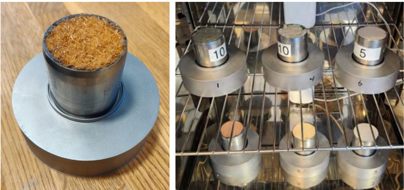
Figure 14: 3D-printed sample holder with bio-based material inside it for Wet/Dry Cup method (left); several Wet/Dry Cup method tests running in the climatic chamber VCL 7010 – Vötsch Industrietechnik [11] (right).
