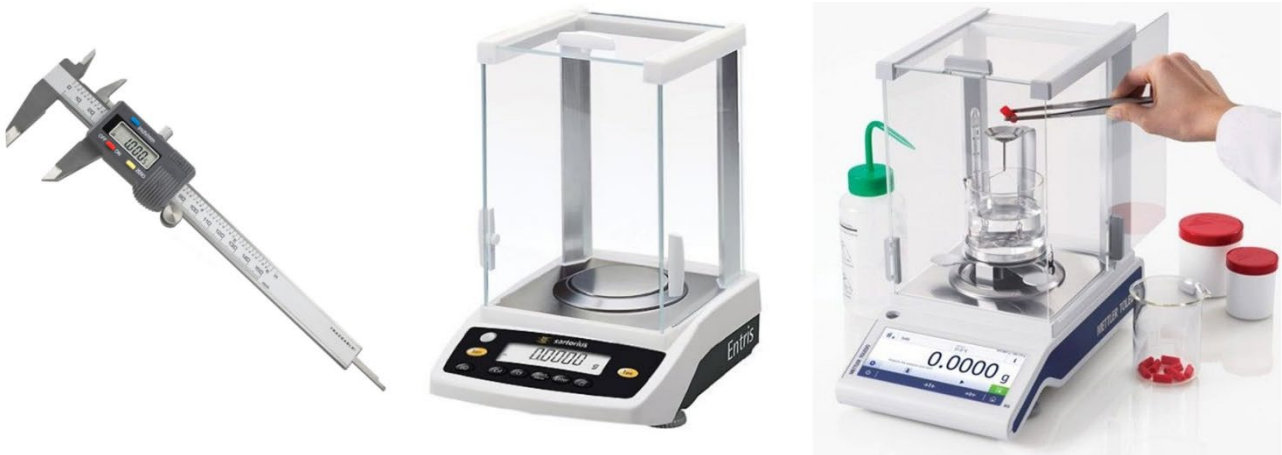
Figure 1: Measurement of dimensions and volume with a precision caliper (left); accurate measurement of mass with a precision scale [3] (center); accurate measurement of the density of small-size samples with the Archimedes' principle of buoyancy on a precision scale [2] (right).
