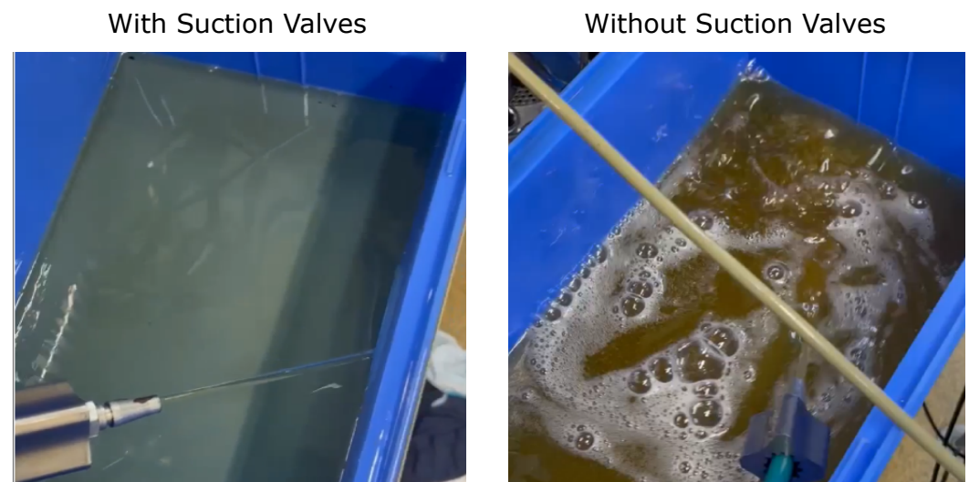
Figure 13. LEFT A picture of the tank oil from the steering unit in the end-stop, with suction valves. RIGHT A picture of the tank oil from the steering unit in the end-stop, where the suction valves are removed.
