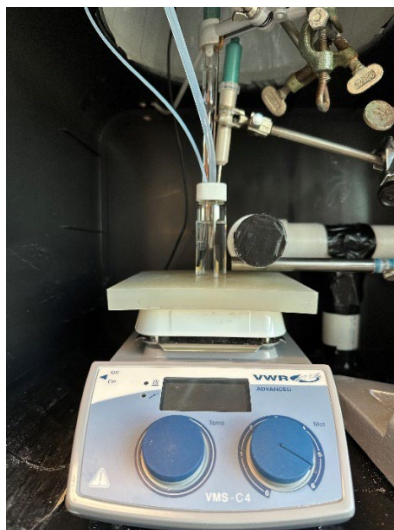
Figure 4-2. Photo of the experimental setup used for measurements of aqueous-phase scavenging reactions at high temperatures (up to 75 °C). Paper B. Reprinted with permission from Ind. Eng. Chem. Res. 2023, 62, 21, 8269–8280. Copyright 2023 American Chemical Society.
