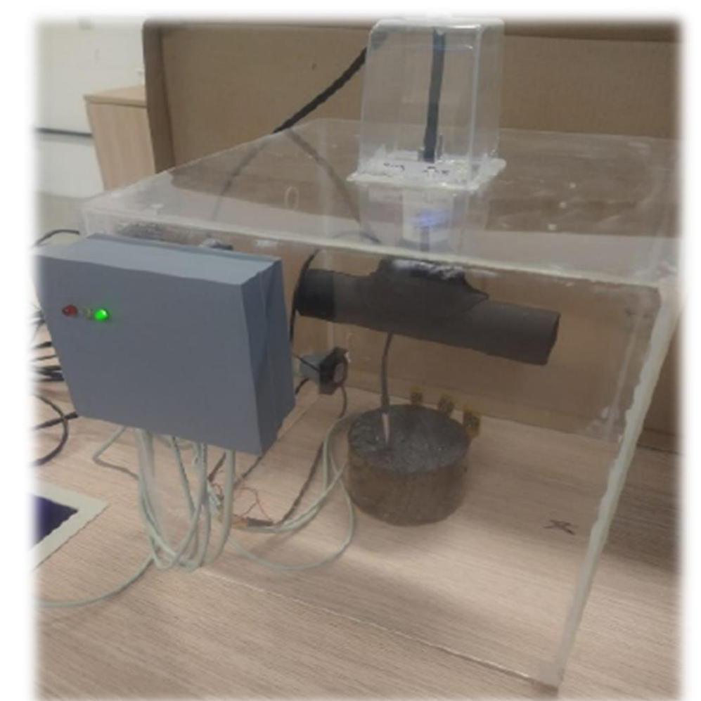
Micro coolers and sensors monitoring environment
